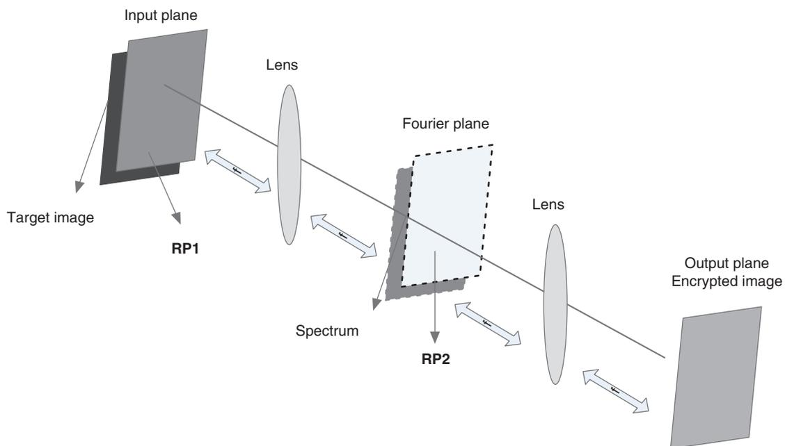
**Figure 1:** The block diagram of the DRPE encryption/decryption
