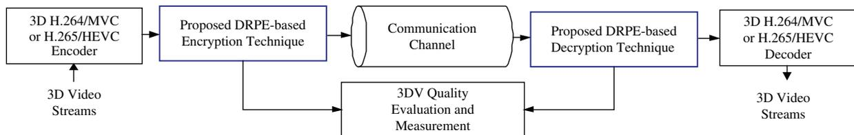
**Figure 2:** The proposed 3DV cybersecurity communication system
