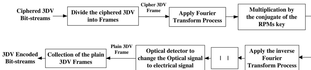
**Figure 4:** The proposed DRPE-based 3DV decryption mechanism
