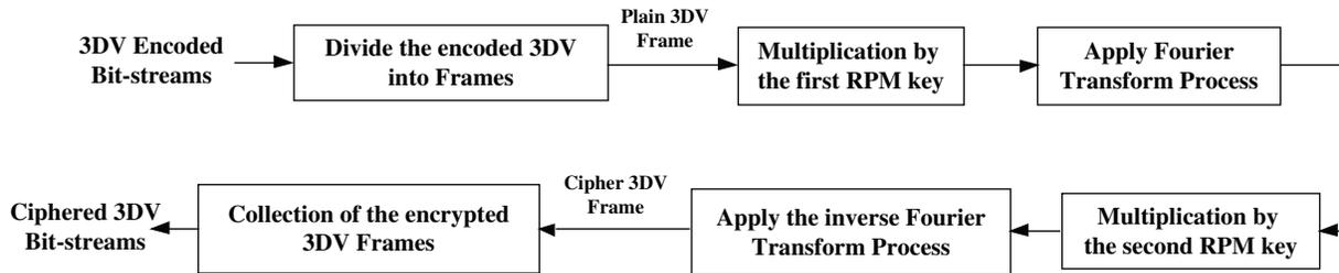
**Figure 3:** The proposed DRPE-based 3DV encryption mechanism
