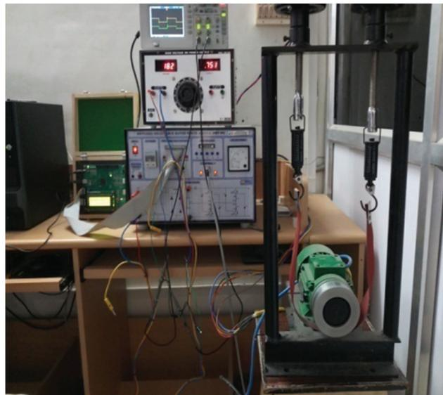
**Figure 7:** The hardware setup of the 8/6 SRM drive
