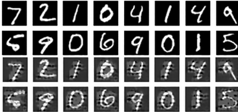
Figure 5: A comparison of clean images and adversarial images. The first two rows are clean images sampled from the MNIST data set, and the last two rows are their corresponding adversarial images produced by our method, which are able to force CM_D to make wrong classification prediction with limited knowledge of the model CM_D
