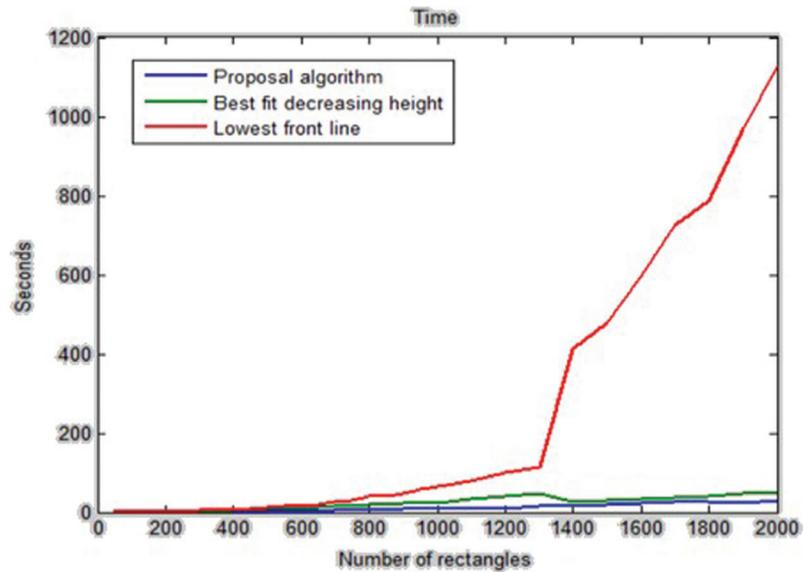
**Figure 4:** The running time of the Best-Fit decreasing height algorithm, the lowest front-line strategy, and the proposed algorithm
