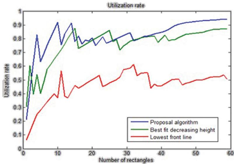
**Figure 3:** The utilization rate of the three Best-Fit decreasing height, the lowest front-line strategy, and the proposed algorithms
