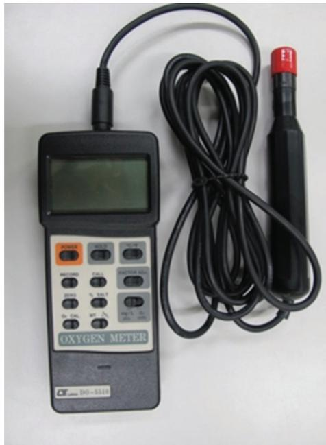
**Figure 7:** Soluble oxygen sensing module
