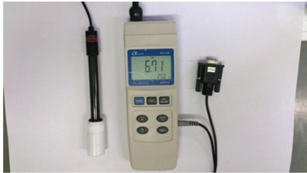
**Figure 10:** pH value sensing module
