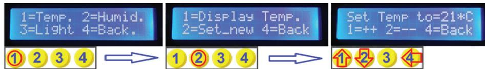
Figure 3: Setting a new desired room temperature
