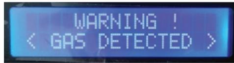
**Figure 13:** The system's LCD notification for gas leak detections
