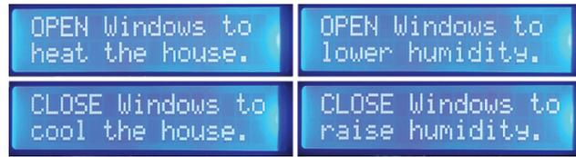
**Figure 10:** Examples of power-saving tips displayed by the system
