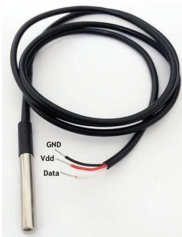
Figure 3: DS18B20 temperature sensor
