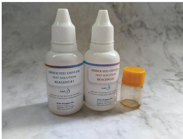
Figure 4: Dissolved oxygen test kit
