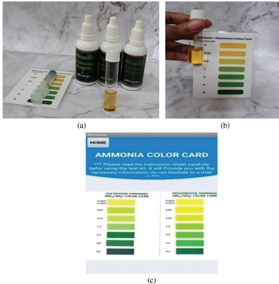
Figure 15: Result of dissolved ammonia, (a) is the solution made by the kit, (b) is the solution with the matching with the provided color code, (c) Shows the interface of the application of the color code
