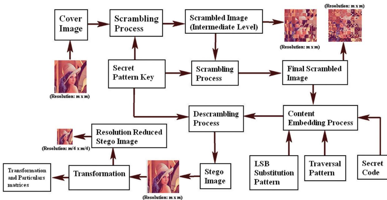
**Figure 5:** Block diagram of scrambling based wavelet transform (SBHWT) approach
