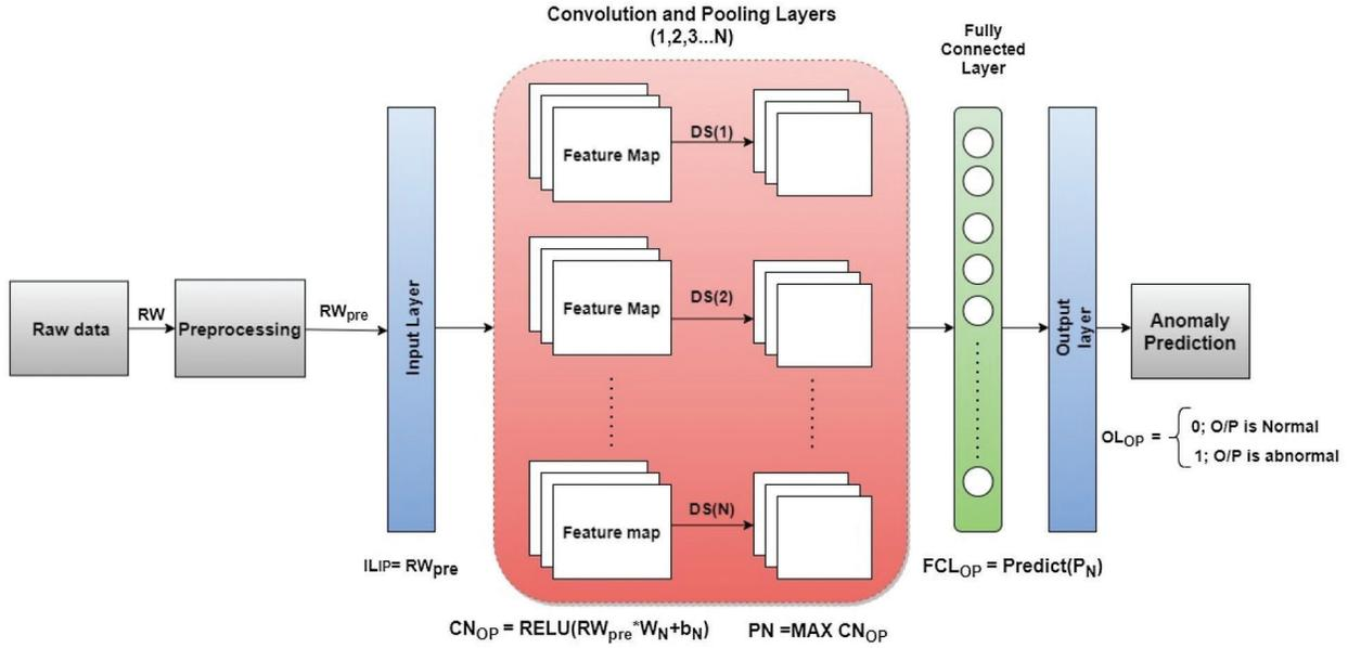
**Figure 2:** Anomaly detection in AV using DL based M-CNN
