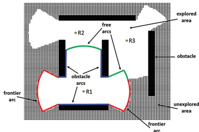
**Figure 2:** Free, frontier and obstacle arcs in exploration
