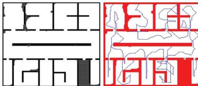
**Figure 7:** The covered area and the path generated by the  $D^*$  Lite algorithm in the environment B with the implemented MCDM-based exploration Strategy 2 (by using TOPSIS)
