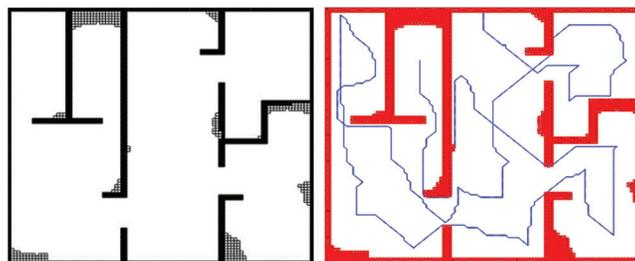
**Figure 6:** The covered area and the path generated by the  $D^*$  Lite algorithm in the environment A with the implemented MCDM-based exploration Strategy 1 (by using TOPSIS)
