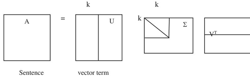
**Figure 3:** SVD skeleton diagram
