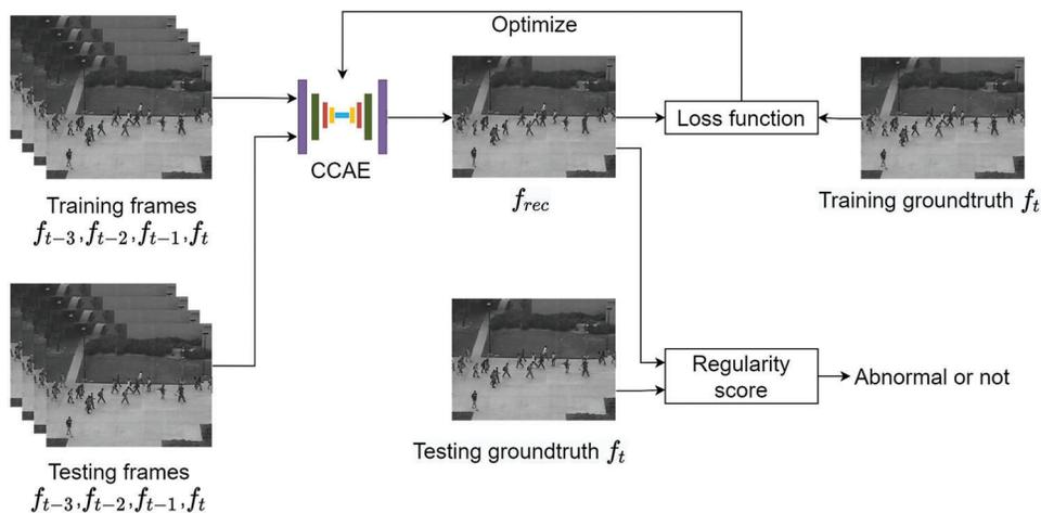
**Figure 1:** The diagram of video anomaly detection process
