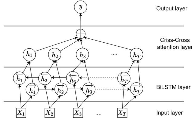
**Figure 4:** The details of CCBiLSTM
