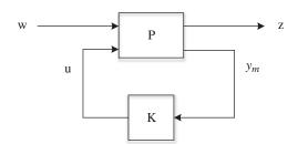
Figure 2: LFT form of the closed-loop system
