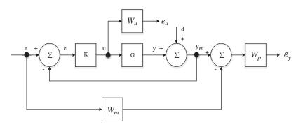
Figure 1: Feedback structure of H-infinity controller
