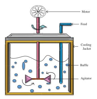
Figure 3: Continuous stirred-tank reactor
