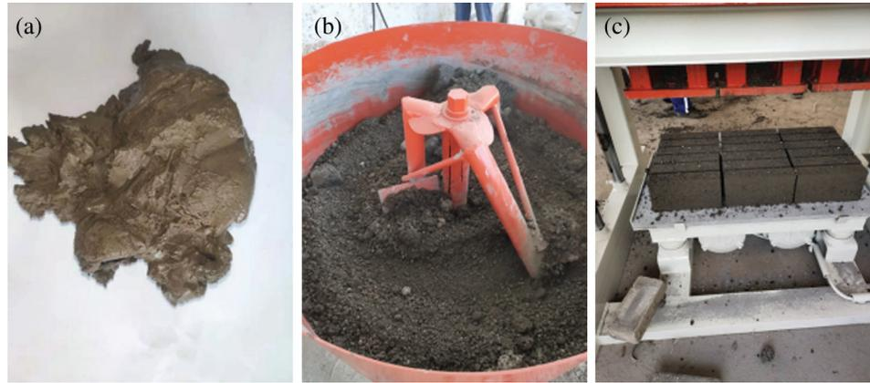
**Figure 9:** (a) OWS; (b) OWS after mixed with solidifying material and recycled aggregates; (c) Non-fired bricks
