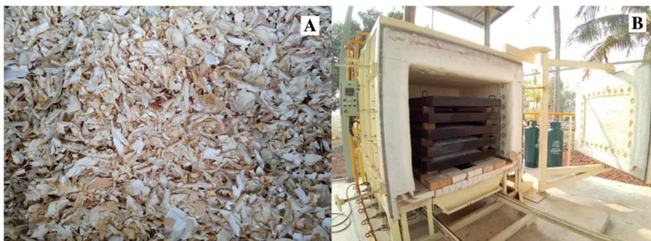
**Figure 1:** Digital images of the dried solid hatchery waste (A) and the industrial car bottom furnace with five stacked trays (B)
