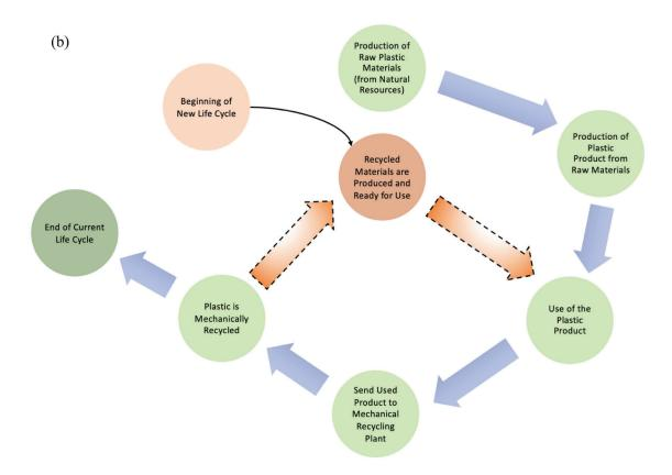
**Figure 3:** A general life cycle of plastic products: (a) A cradle-to-grave life cycle where disposal of plastic product is the end of the life cycle; (b) A cradle-to-cradle life cycle where recycling of plastic product is an option (the life cycle adapts to having a re-used input of materials)
