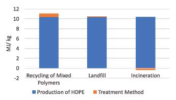
Figure 7: Additional energy uses for the three disposal methods on top of the production of 1 kg of HDPE
