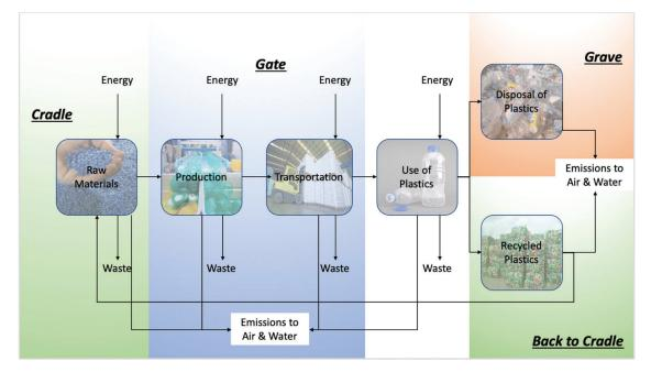
**Figure 1:** A Life Cycle Analysis (LCA) is differentiated amongst several parts, including cradle, gate, and grave. If the recycling process is to be evaluated, the product would be generated from the cradle and would be sent back to the cradle for production again
