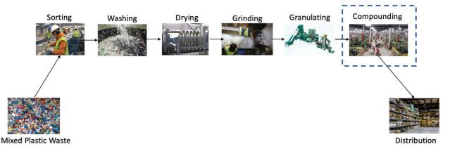
**Figure 5:** Network of the recycling of mixed polymers process (mechanical recycling, adapted from [22]). It should be noted that SimaPro 7.1 does not include compounding as part of the recycling of mixed polymers process; realistically, this step is included in mechanical recycling
