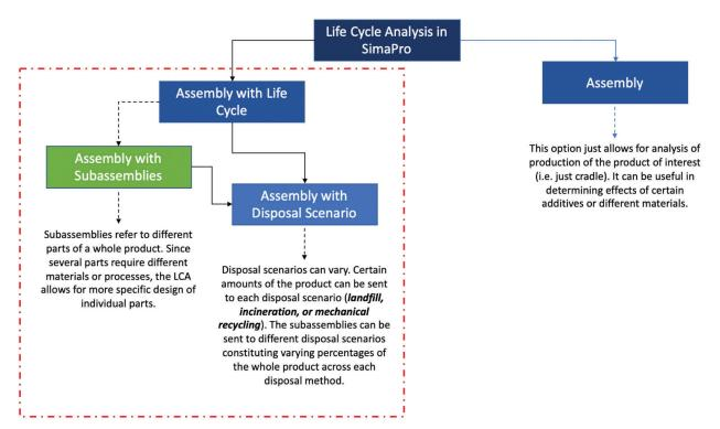
**Figure 2:** General stepwise process of creating an LCA in SimaPro 7.1. The left-hand side refers to the option that was chosen for this analysis. *Assembly with subassemblies* is an additional option provided in the constructing of this method, allowing for more specific analysis. The right-hand side is just analyzing the production of the product of interest and was not used for this analysis because of a lack of a disposal scenario
