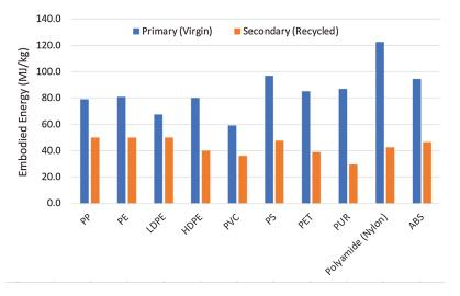
**Figure 4:** Various embodied energies of primary (virgin) and secondary (recycled) plastics (modified from the REMADE calculator) [20]
