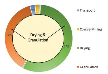
**Figure 8:** Breakdown of fossil fuel usage for mechanical recycling of mixed polymers. Drying and granulation use the most energy in the 11-step process. Other steps include transport (2.35%), shredding (0.093%), course milling (1.86%), separation in fluid tank (0.028%), fine separation in hydrocyclon (0.037%), water separation in spin drier (0.42%), fine milling (0.33%), ultra-fine cyclone separation (0.42%), and internal transport (0.046%)
