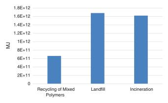
**Figure 9:** Analysis of the energy requirements for all the HDPE (59.5 million tons) that is produced annually to undergo three life cycles for each respective disposal scenario
