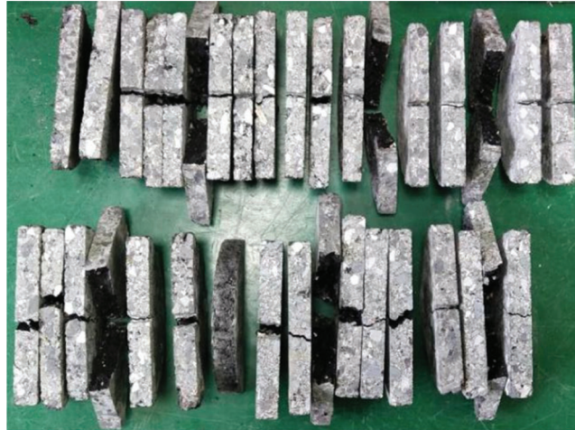
Figure 8: Part of the specimen after SCB test
