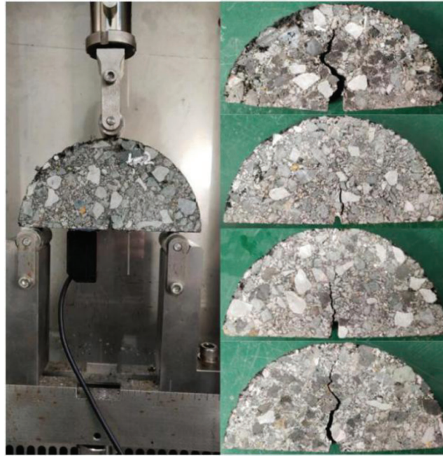
Figure 4: Set-up of semi-circular bend test and loaded specimens
