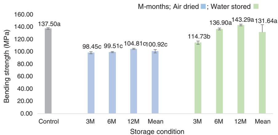
**Figure 9:** Bending strength variations of *P. edulis* culms under different storage conditions
