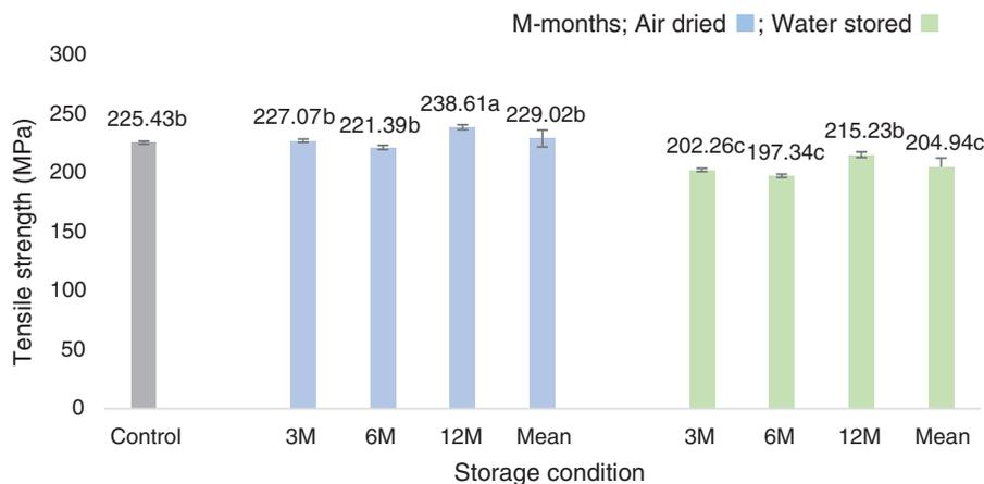
**Figure 10:** Tensile strength variations of *P. edulis* culms under different storage conditions
