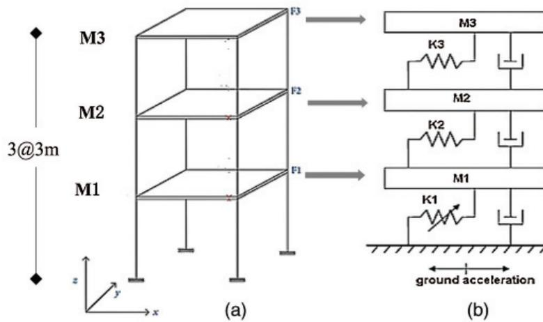
**Figure 3:** Analytical model. (a) Model of a three-story frame structure (b) Spring-mass-damper model
