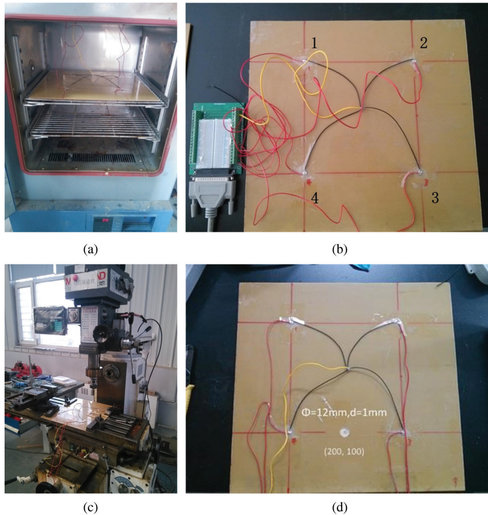
Figure 4: Experiments setup of damage diagnosis on composite plate under variable temperature environment. (a) The oven with the specimen (b) The specimen with 4 sensors (c) The Miller and specimen (d) The specimen with a countersink
