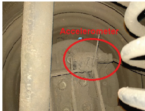
Figure 5: MEMS Accelerometer fixed on the axle
