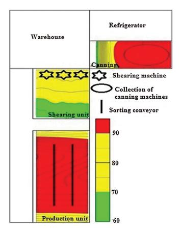
Figure 1: Noise-isosonic map of canning, production and shearing units by Surfer software
