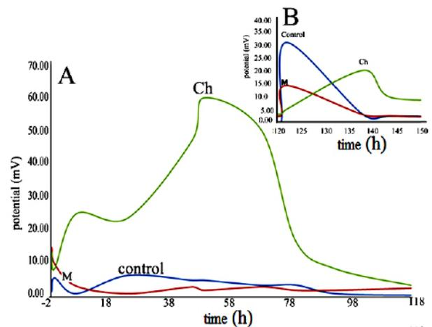
**FIGURE 2.** Electrochemical behavior of PVA-H (control), PVA-H-*C. vulgaris* (Ch), and PVA-H-*M. reisseri* (M) composites. A: from the beginning of the experiment; B: after addition of 1 ml water to each composite.
