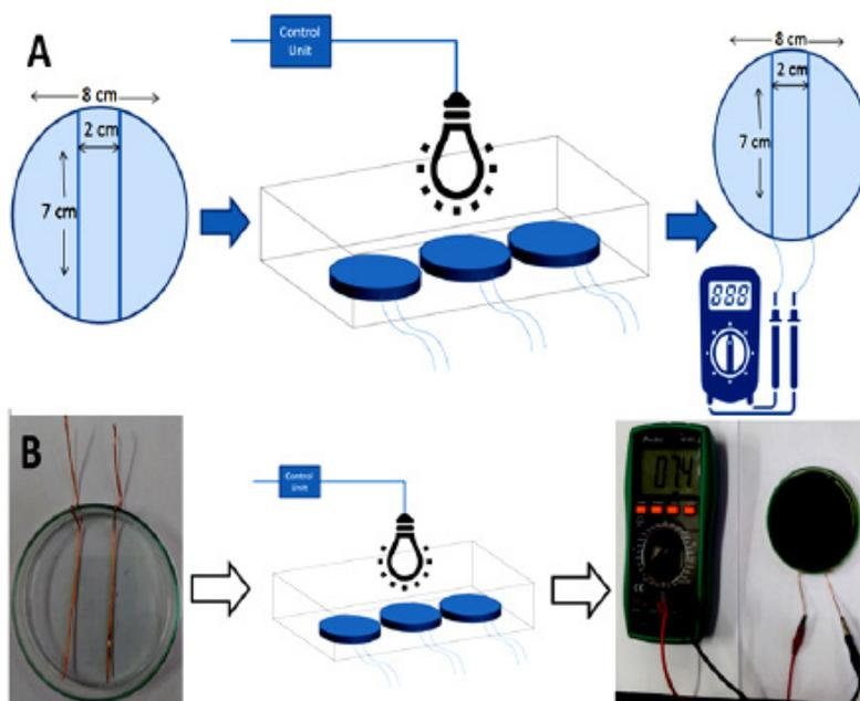
FIGURE 1. Laboratory designed algal solar cells. A. diagrammatic illustration of the design. B. the actual system.
