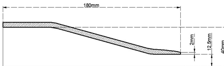
**Figure 2:** Nozzle geometry of axisymmetric jet flow
