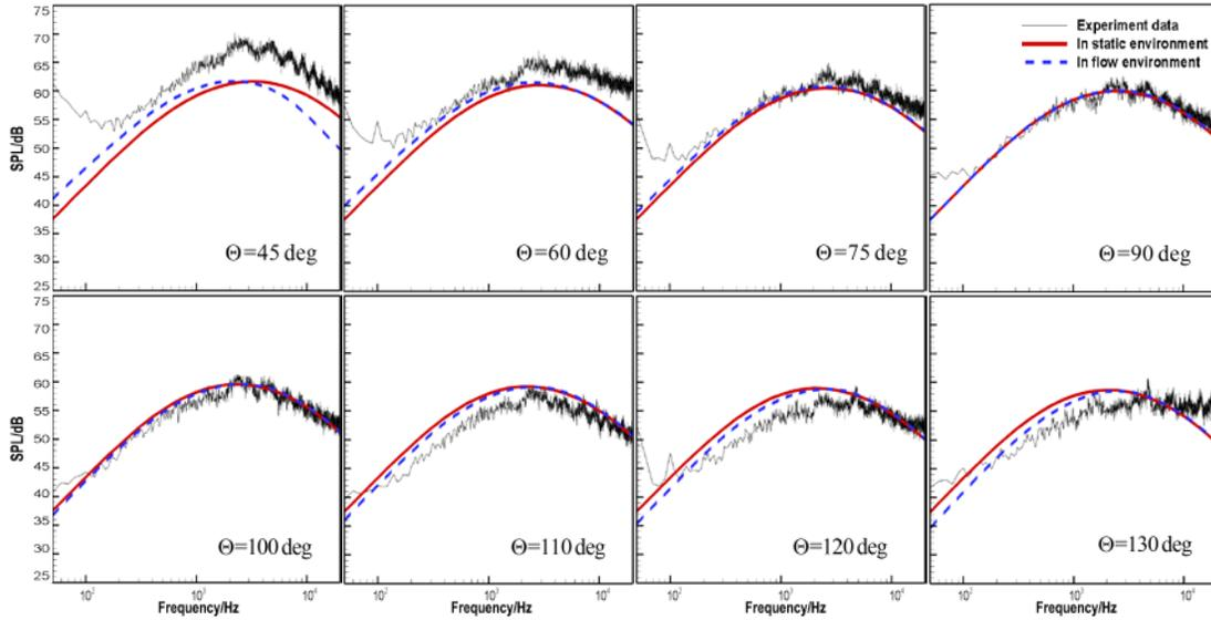
**Figure 9:** Predictions compared with measurement for the  $M_j = 0.9$
