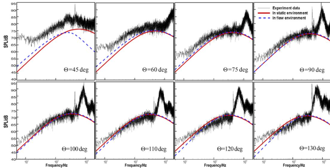
**Figure 11:** Predictions compared with measurement for the  $M_j = 1.5$
