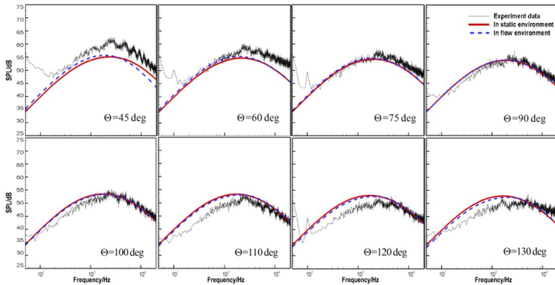
**Figure 8:** Predictions compared with measurement for the  $M_j = 0.7$
