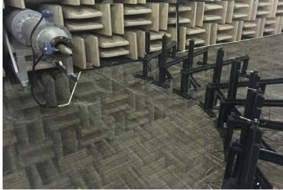
**Figure 6:** The photograph of the microphone array
