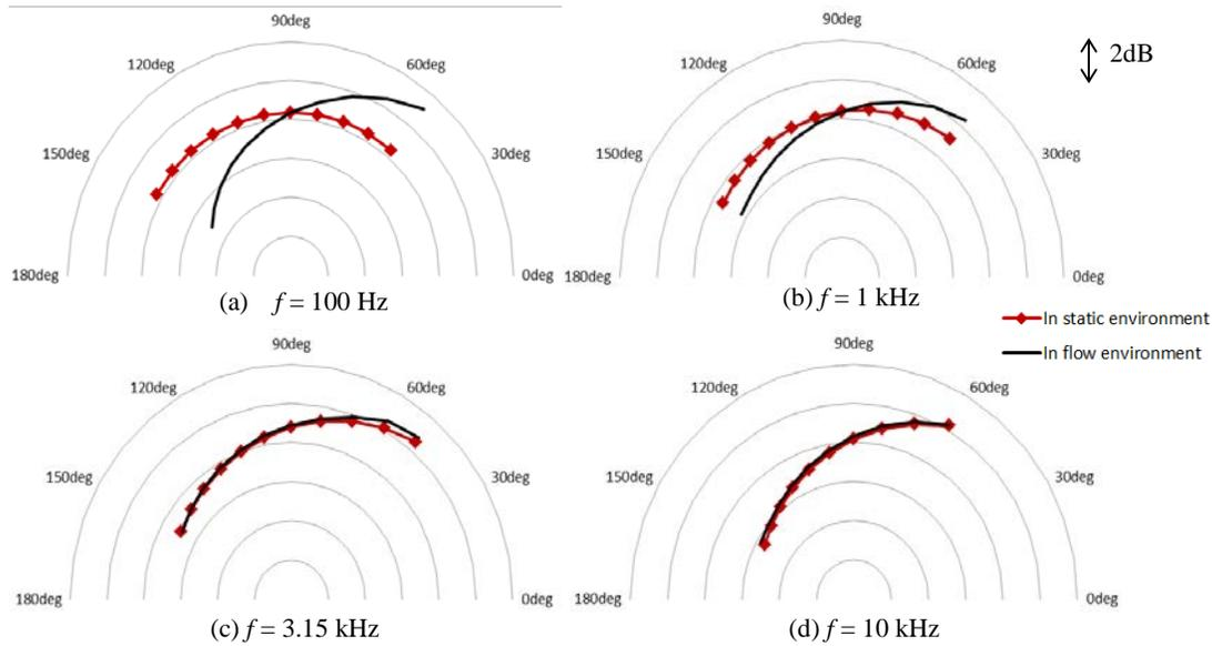
**Figure 4:** Comparisons between the directivity of sound source in static and flow environments
