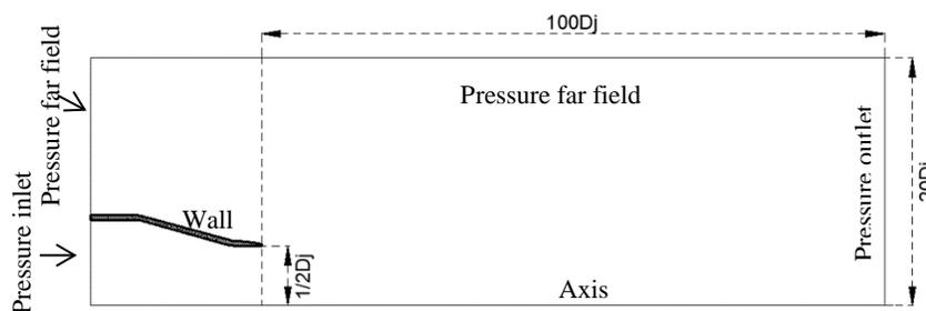
**Figure 3:** The schematic of computation domain
