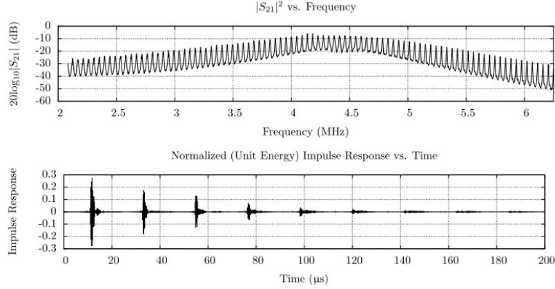
**Figure 2:** Measured characteristic of a communication channel (transducer center frequency at 4 MHz, 6.35-cm thick steel plate: [top] power transfer function ( $|S_{21}|^2$ ) and [bottom] band-limited impulse response (2.08 MHz-6.25 MHz)
