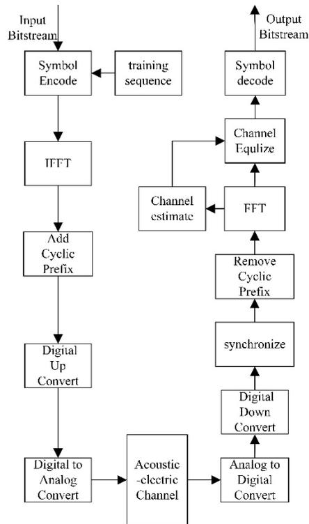
**Figure 5:** The architecture of the OFDM-based ultrasonic wireless communication system through metal barriers
