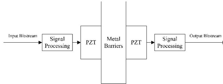
**Figure 1:** The sandwiched structure in an ultrasonic wireless communication system through metal barriers
