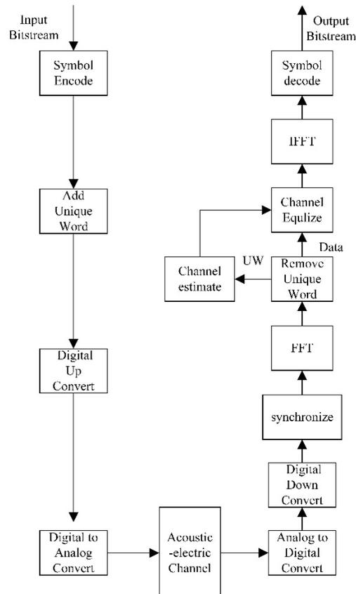
**Figure 6:** The architecture of the SC-FDE based ultrasonic wireless communication system through metal barriers
