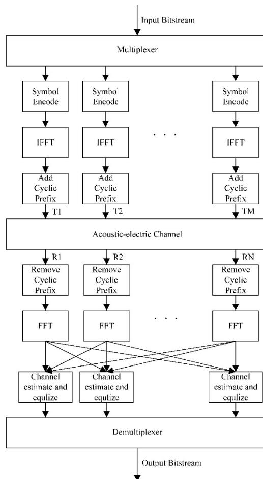
**Figure 7:** The architecture of the MIMO-OFDM ultrasonic wireless communication system through metal barriers
