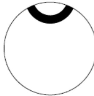
**Figure 4:** Transducer face asymmetry due to wrap electrode
