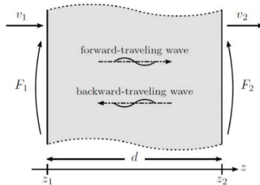
**Figure 3:** The dual-port network of a semi-infinite elastic material
