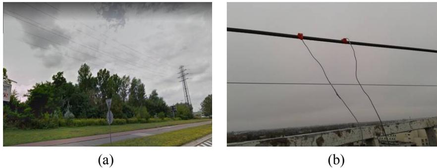
**Figure 3:** Experiments in situ, (a) view of the overhead transmission line (b) accelerometers mounted to the transmission conductor
