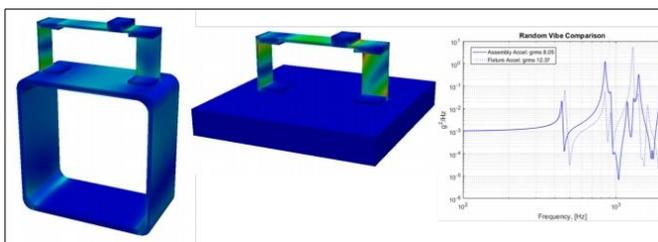
Figure 2. Component testing boundary condition problem, random vibration (simulation) example. Stress field from random input to the base of the assembly (l.). Component stress field from acceleration input at the base of the component, derived from the assembly response (center.) Assembly response vs component response on fixture, derived using traditional techniques (r.) From the presentation at IMAC 35.
