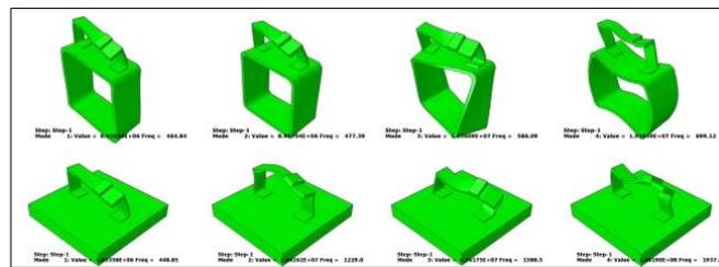
Figure 3. First four flexural modes from Finite Element Models of the component-in-assembly and component-on-fixture configurations, steel, free boundary conditions.
