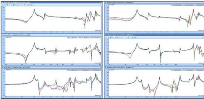
Figure 6. Single bolt attachment (l.) vs. Four bolt attachment (r.) at a driving point (top plot) and two additional response locations. Once the initial data set was taken, the component was removed and re-attached to the assembly twice, with the same measurements repeated after each re-attachment.
