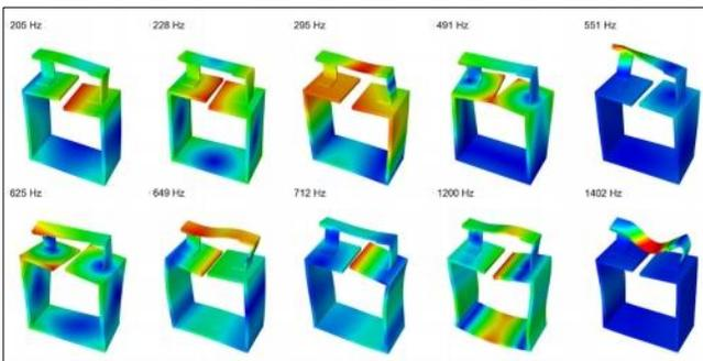
Figure 8. Flexural mode shapes of the final design, from a finite element model.
