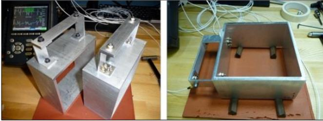
Figure 5. Impact survey on Single vs Four bolt attachment.
