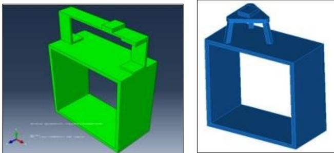
Figure 1. Component concepts: C-channel vs. three-leg designs.
