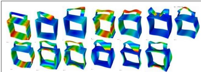
Figure 7. Uncut Aluminum Box Assembly flexural mode shapes from modeling.
