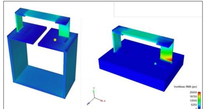
Figure 9. Component testing boundary condition problem simulation for random vibration. Random acceleration input was applied to the base of the assembly. The stress field (color contours) and response at the component base (indicated by a yellow dot) was calculated (l.). Component stress field from acceleration input at the component base (indicated by a green dot), derived from the assembly response (r.).
