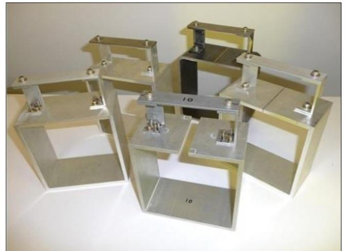
Figure 10. Development prototypes, and the final version (front) of the Box and Bench test bed for the component test boundary condition problem.
