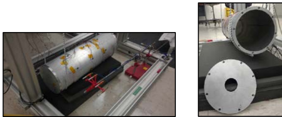
Figure 2. Experimental test setup. Right: Cylinder suspended from soft bungee cords with the accelerometers bonded on the outer surface, and the microphones distributed in an array. Left: Hollow cylinder with end cap removed.
