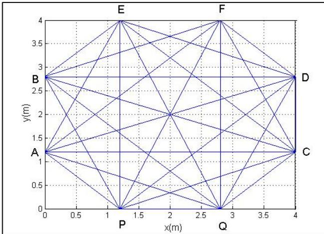
Figure 1. Arrangement of transceivers and division of the measure area.
