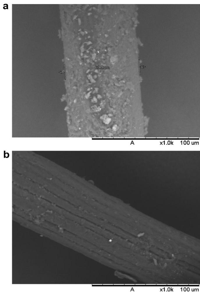
**Figure 5:** Untreated (a) and treated (alkaline treatment) (b) date palm fiber [98]. Permission obtained through Rights Link®
