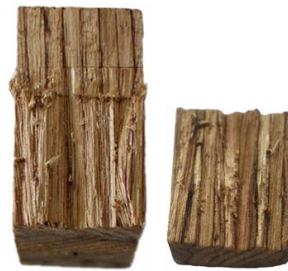
Figure 11: Typical failure mode of specimens in shear tests
