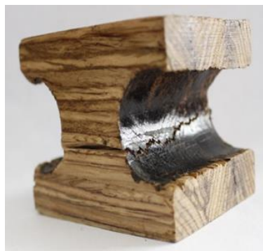
Figure 6: Typical failure mode of specimens in perpendicular-to-grain tensile tests
