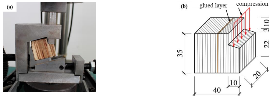
Figure 10: Shear test: (a) setup; (b) specimen geometry
