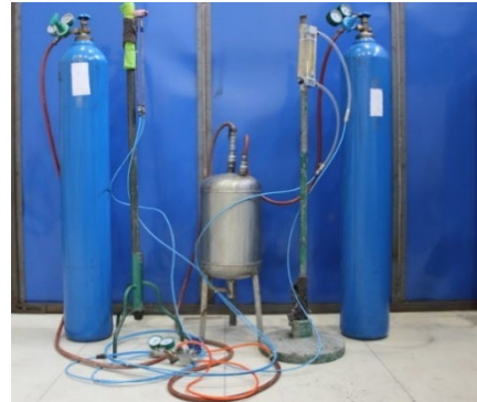
Figure 4: Multi-component two phase flow water mist fire extinguishing system
