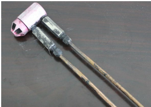
Figure 3: Two phase flow water mist fire extinguishing nozzle
