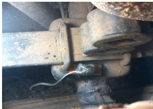
Figure 5: MEMS accelerometer fixed on the axel
