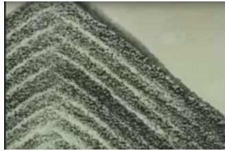
Figure 9: Experimental lamination of a heterogeneous mixture of two sands that differ in density and grain-diameter
