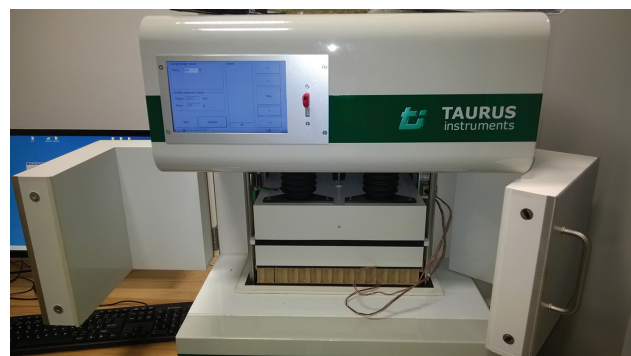
Figure 3 The TLP 300 DTX-1 thermal conductivity measuring device.
