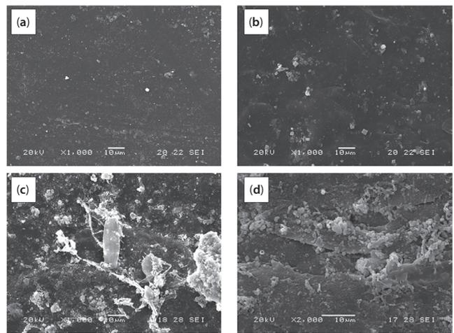
Figure 7 SEM micrographs of film surface of PE (a), PE/20HC1 (b) and PE/20HC2 (c,d) retrieved from marine environmental test flasks after 54 weeks of incubation.
