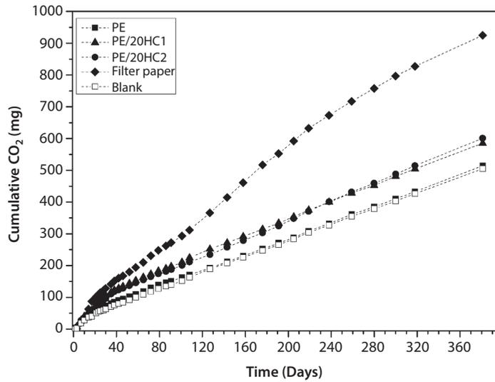
Figure 6 Cumulative CO<sub>2</sub> emissions of PE/HCs, PE, filter paper and blank in marine environment test.
