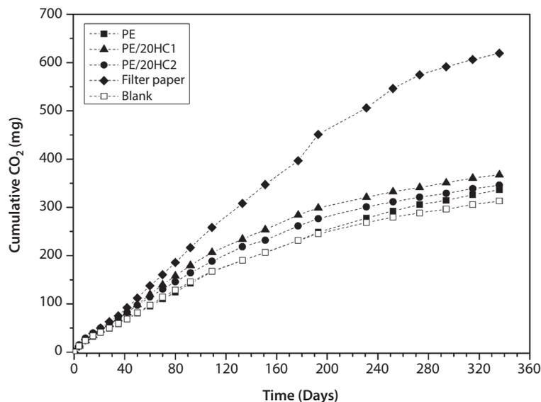
Figure 3 Cumulative  $\text{CO}_2$  emissions of PE/HCs, PE, filter paper and blank in terrestrial respirometric test.
