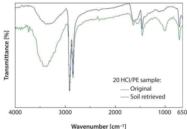
**Figure 5** FTIR spectra of PE/20HC1.
