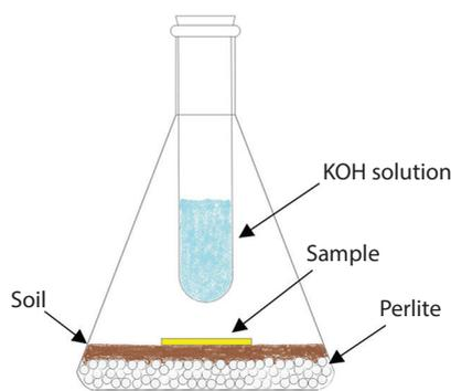
Figure 1 Flask for terrestrial biodegradation test.
