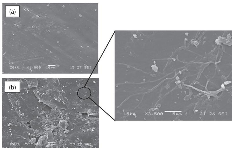
**Figure 4** SEM micrographs of film surface of PE/20HC1 (a) and PE/20HC2 (b) retrieved from terrestrial respirometric test flasks after 48 weeks of incubation.
