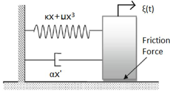
**Figure 1:** Schematic of friction system with random excitation
