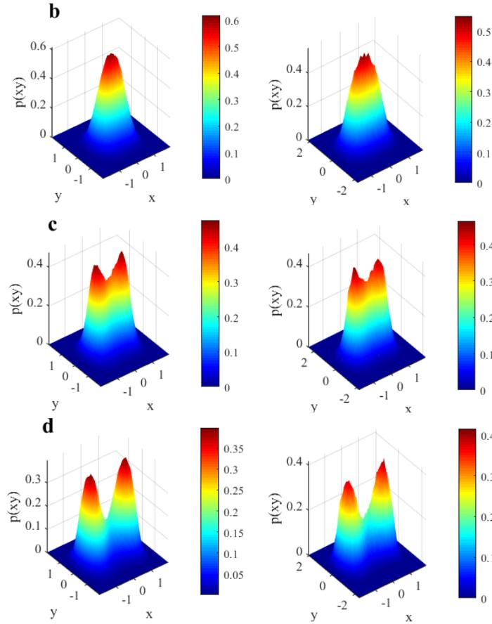
**Figure 5:** The steady-state joint PDFs of system (9) with  $\alpha = 0.5, 0, -0.5, -1$ . Left sides: the SGCM method results; right sides: MC simulation method results. (a)  $\alpha = 0.5$ ; (b)  $\alpha = 0$ ; (c)  $\alpha = -0.5$ ; (d)  $\alpha = -1$
