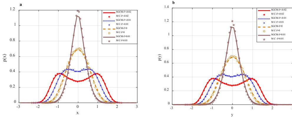
**Figure 2:** The steady-state marginal PDFs of system (6) with  $f_c = -0.02, -0.01, 0, 0.01$ . (a) The steady-state marginal PDFs of  $x$ ; (b) The steady-state marginal PDFs of  $y$ . Solid lines: the SGCM method results; symbols: MC simulation method results
