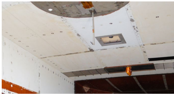
Figure 6: Prandtl pitot probe for the blockage correction
