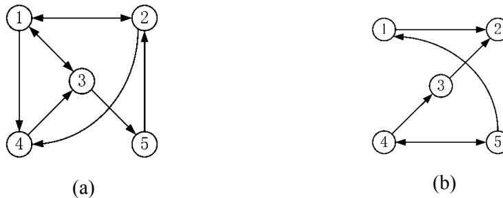
Figure 1: Interaction topologies: (a) G_1 and (b) G_2 . An arrow from node j heading to node i implies agent i receives information of agent j ; thus j is a neighbor of i . Both G_1 and G_2 have a directed spanning tree
