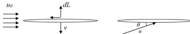
Figure 5: Schematic of wing model and incoming flow
