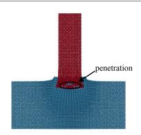
**Figure 12:** Non-physical penetration occurring in the case of using CSLH=1.1 for SPH with PCM
