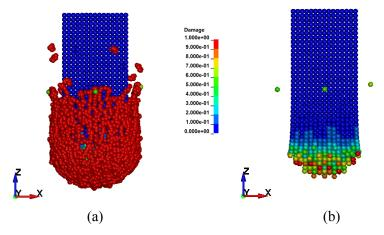
**Figure 3:** Residual mass prediction: (a) Simulated whole projectile; (b) Projectile after removing damaged particles
