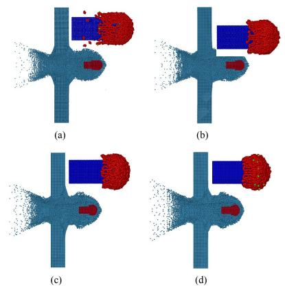
**Figure 13:** Deformations of projectile and target at 60 µs obtained by SPH with PCM: (a) CSLH=1.2; (b) CSLH=1.3; (c) CSLH=1.4; (d) CSLH=1.5
