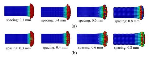
**Figure 8:** Simulated deformations of the projectile at 8 µs after impact using different particle spacings: (a) SPH with PCM; (b) SPH with PAM
