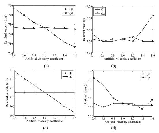
**Figure 9:** Effects of artificial viscosity coefficients on residual velocity and mass: (a) Residual velocity for PCM; (b) Residual mass for PCM; (c) Residual velocity for PAM; (d) Residual mass for PAM
