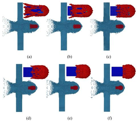
**Figure 14:** Deformations of projectile and target at 60 µs obtained by SPH with PAM: (a) CSLH=1.0; (b) CSLH=1.1; (c) CSLH=1.2; (d) CSLH=1.3; (e) CSLH=1.4; (f) CSLH=1.5
