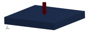
**Figure 1:** SPH model for an Al<sub>2</sub>O<sub>3</sub> ceramic tile normally impacted by a blunt tungsten heavy alloy projectile
