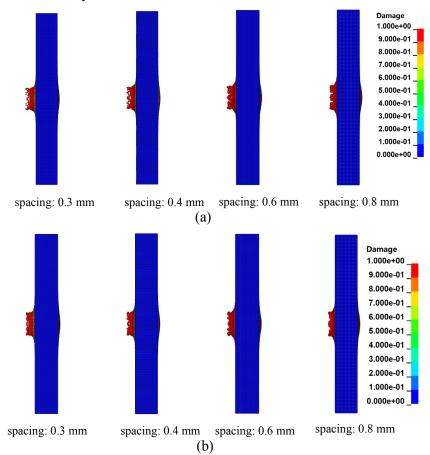
**Figure 5:** Simulated deformations of the target at 10  $\mu$ s after impact using different particle spacings: (a) SPH with PCM; (b) SPH with PAM
