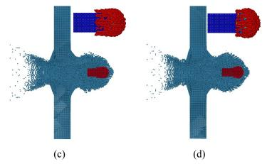
**Figure 10:** Deformations of projectile and target at 60  $\mu$ s obtained by SPH with PCM: (a)  $Q_2=0.4$ ; (b)  $Q_2=0.8$ ; (c)  $Q_2=1.2$ ; (d)  $Q_2=1.6$
