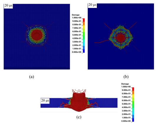
Figure 6: Damage contour of the target: (a) Front view; (b) Back view; (c) Section view
