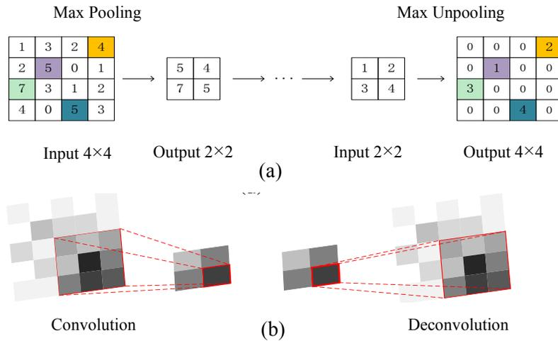
**Figure 3:** Comparison of anti-pooling and deconvolution
