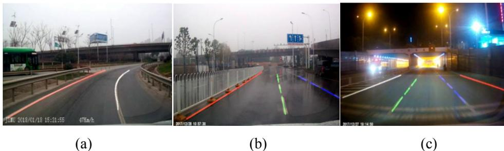
**Figure 7:** Test results in different environments: (a) Test results of curved road sections; (b) Test results of rainy days; (c) Test results of night
