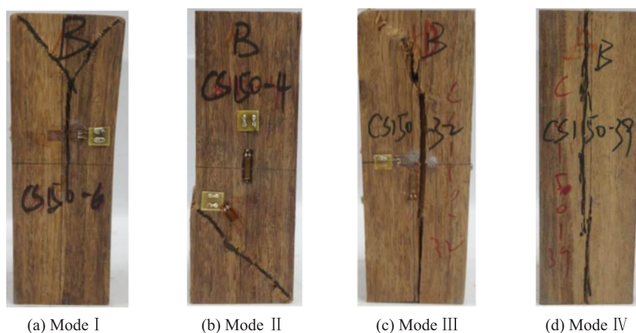
Figure 9: Typical failure modes for axial compression specimens
