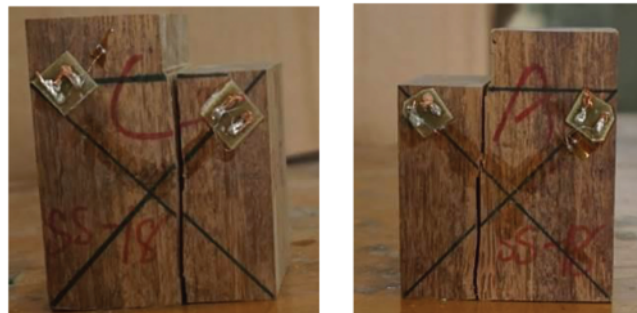
Figure 12: Typical failure mode for shear specimens
