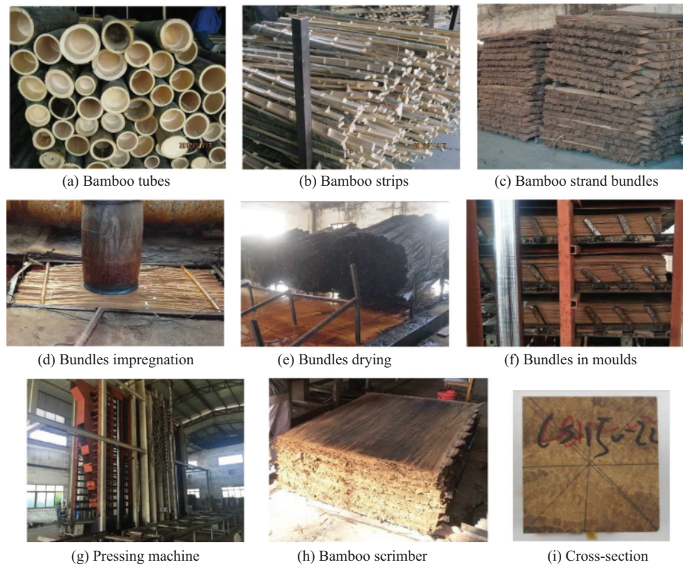
Figure 1: Main manufacturing process for bamboo scrimber
