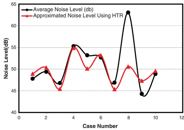
**Figure 18:** Comparison of measured average noise level with approximated noise level using Eq. (15)
