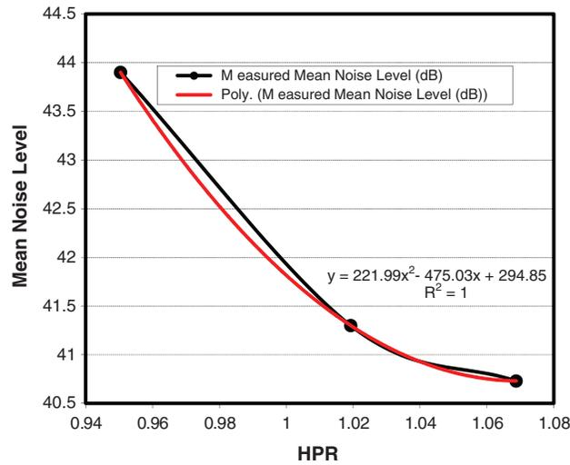
**Figure 11:** Measured mean noise level against non-dimensional value HPR
