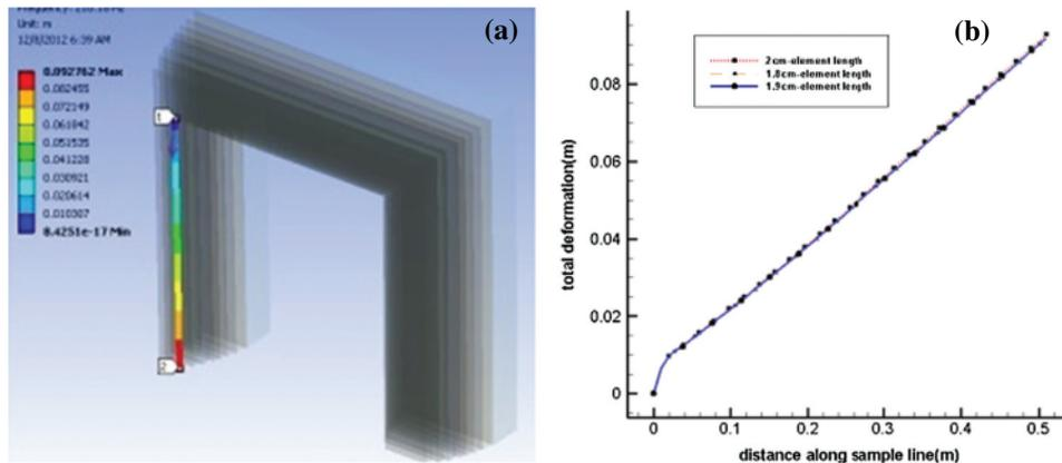
**Figure 6:** (a) Sample edge for deformation evaluation, (b) grid independency graph
