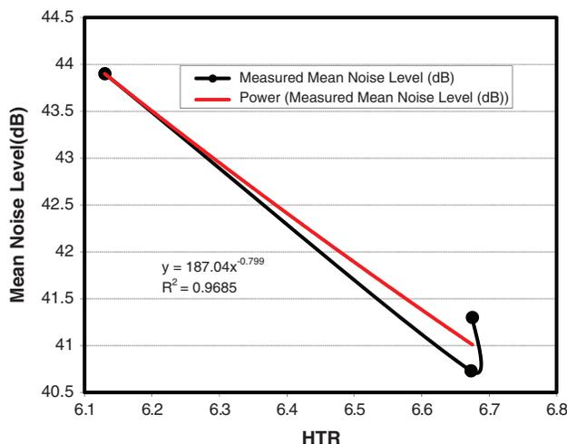
**Figure 12:** Measured mean noise level against non-dimensional value HTR
