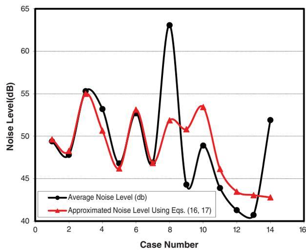
**Figure 19:** Comparison of measured average noise level and approximated noise level using Eqs. (16, 17)
