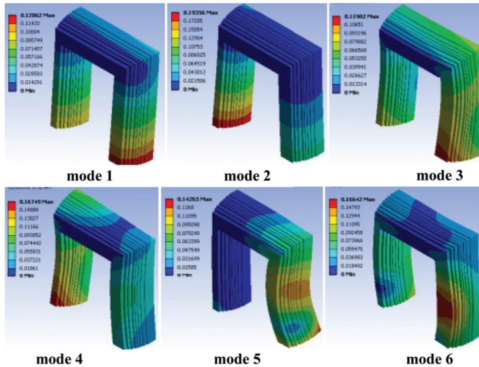
**Figure 8:** First six mode shape of vibration-case5
