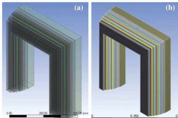
**Figure 4:** (a) The 1/8-fraction of the 3-phase transformer core, (b) model ready for simulation in ANSYS
