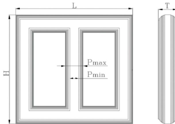
**Figure 2:** Main dimensions of the core
