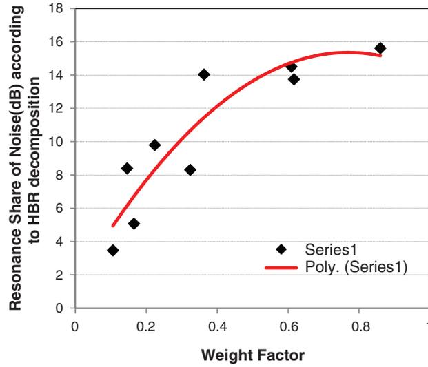
**Figure 13:** Resonance share of Noise according to HBR decomposition against frequency weight factor
