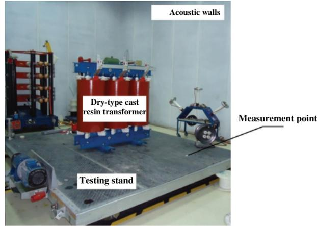
**Figure 1:** Test-rig for noise value evaluation due to IEC60651
