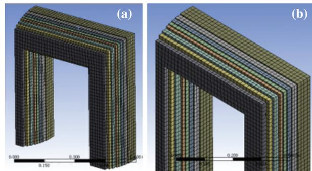
**Figure 7:** (a) Final grid that is used for simulation, (b) exaggerated view of generated mesh
