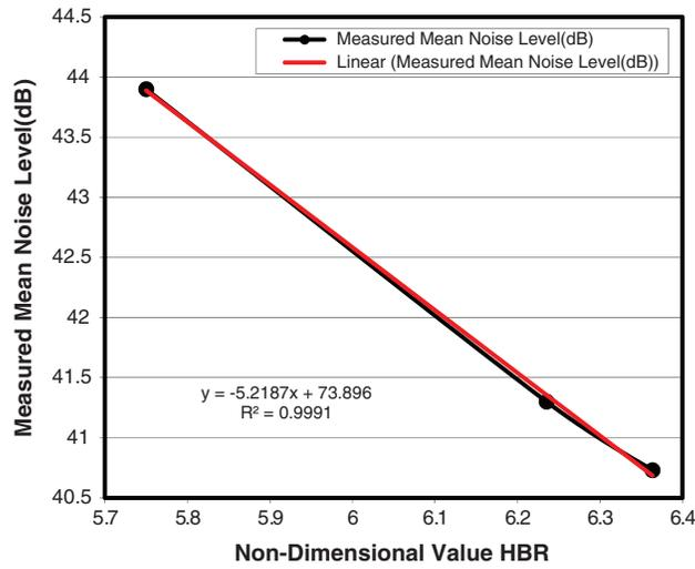
**Figure 10:** Measured mean noise level against non-dimensional value HBR
