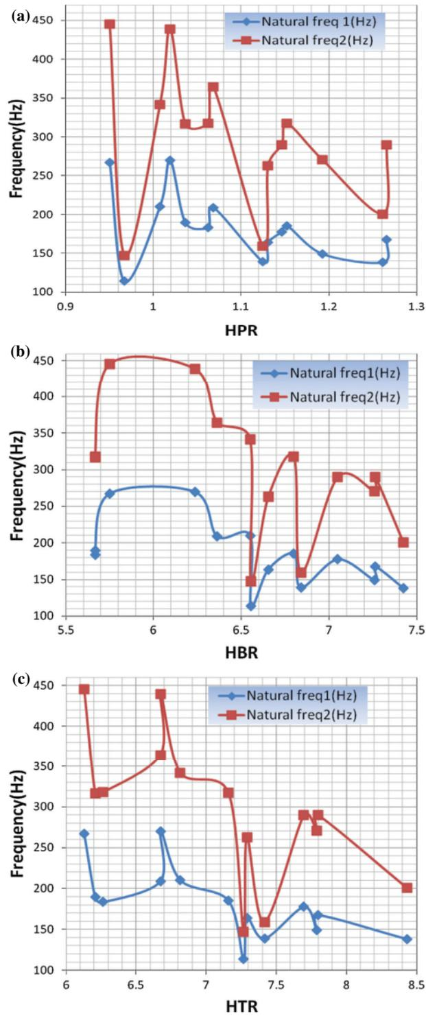
**Figure 9:** First and second natural frequencies of the transformer core against non-dimensional geometrical values (a) “HPR”, (b) “HBR”, (c) “HTR”
