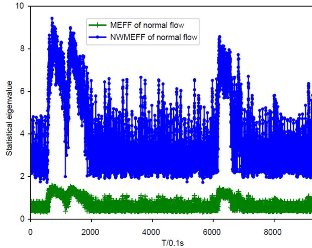
**Figure 3:** Statistical eigenvalue of MEFF and NWMEFF in normal flow
