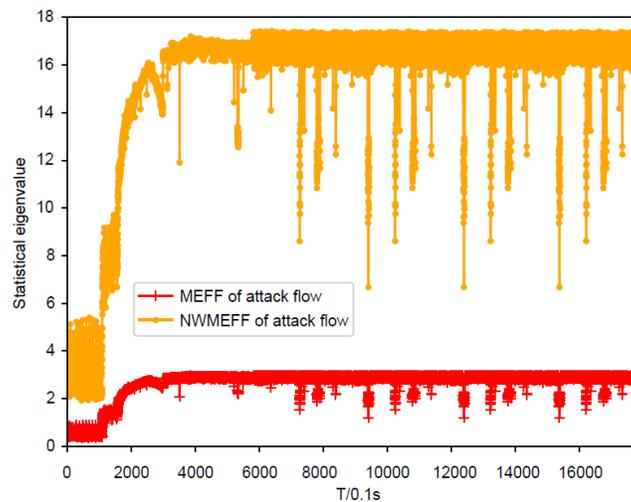
**Figure 4:** Statistical eigenvalue of MEFF and NWMEFF in attack flow
