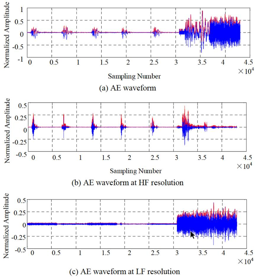
Figure 3: AE from coal at three different resolutions
