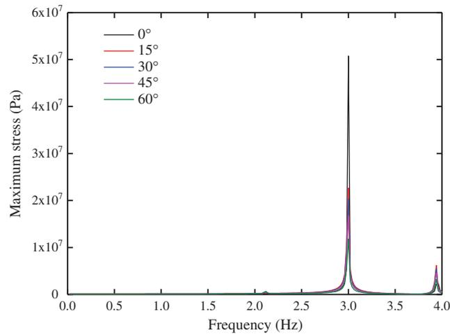
**Figure 22:** Maximum stress at different load angles
