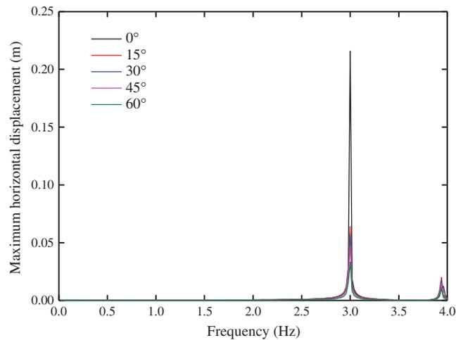
**Figure 20:** Maximum horizontal displacement at different load angles
