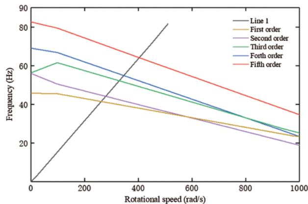
**Figure 6:** Frequency excited by rotational speed and natural frequency
