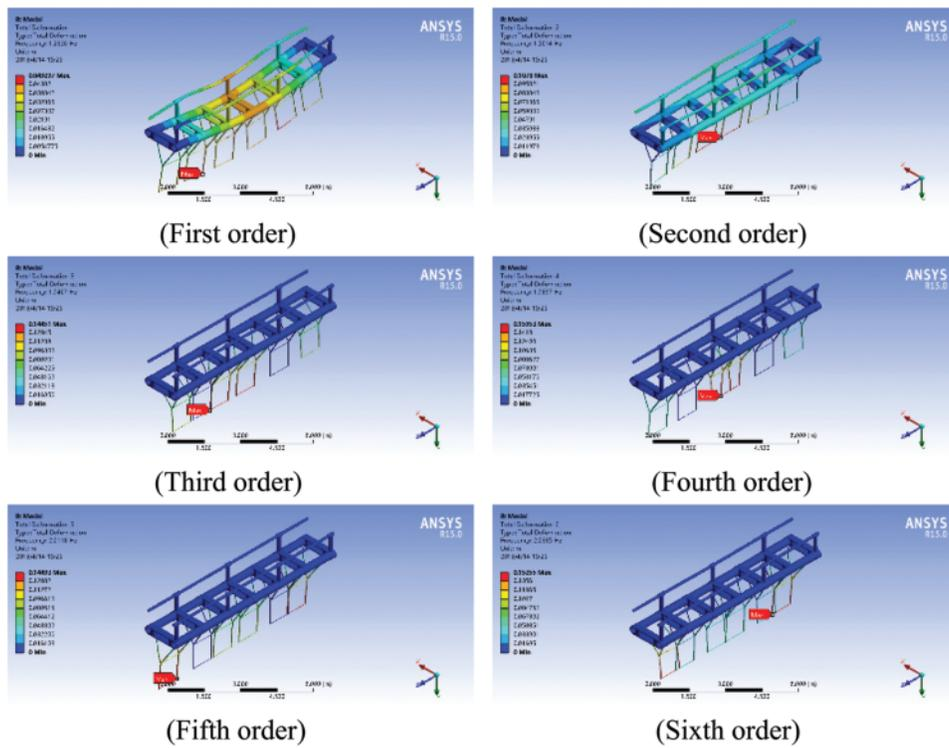
Figure 12: The first six modes of the six units structure
