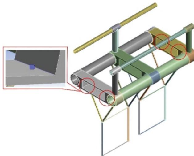
**Figure 7:** Fixed constraint of four anchor points
