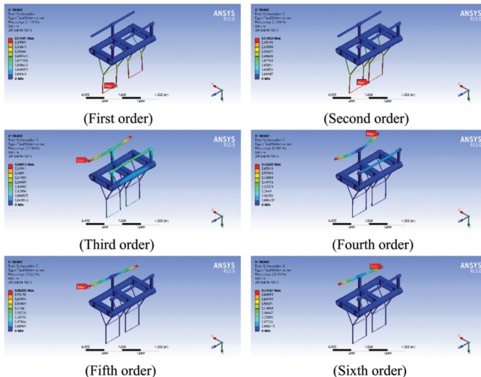
**Figure 8:** The first six mode shapes of two units structure
