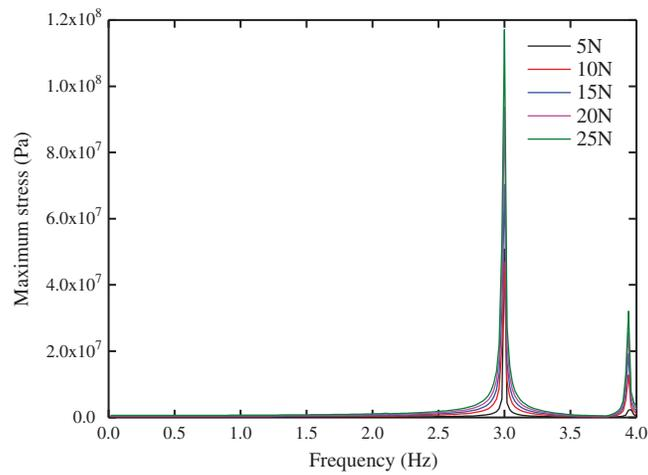
**Figure 19:** Maximum stress at different load angles
