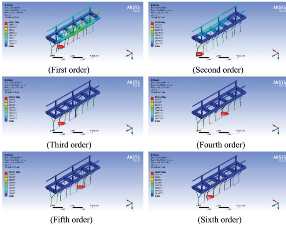
Figure 11: The first six mode shapes of five units structure
