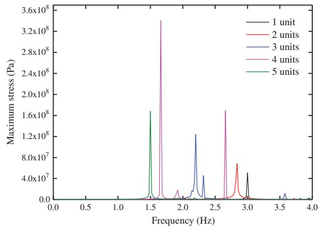
**Figure 16:** Maximum stress for different stent lengths
