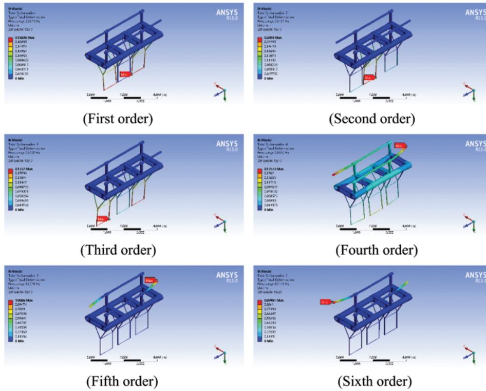
Figure 9: The first six mode shapes of three units structure
