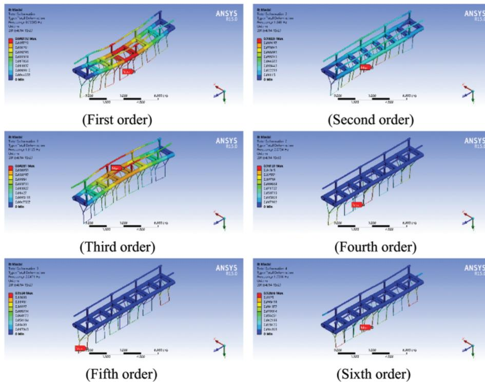
**Figure 13:** The first six mode shapes of seven units structure
