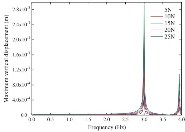
**Figure 18:** Maximum vertical displacement at different load amplitudes
