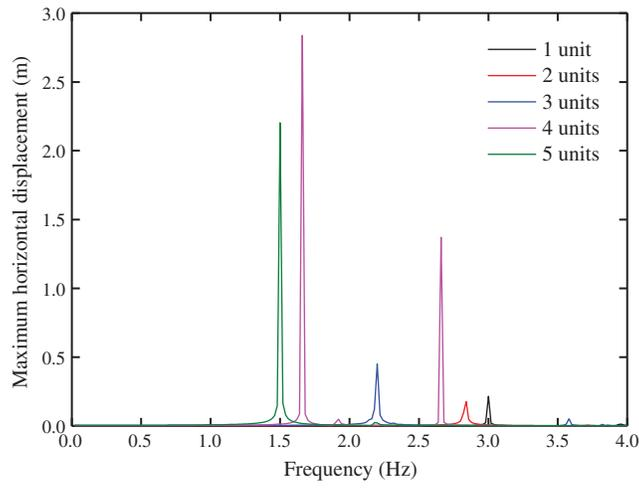
**Figure 14:** Maximum horizontal displacement for different stent lengths
