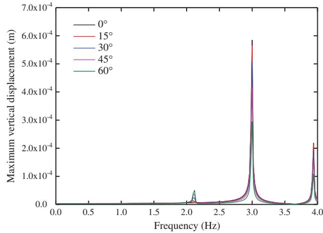
**Figure 21:** Maximum vertical displacement at different load angles
