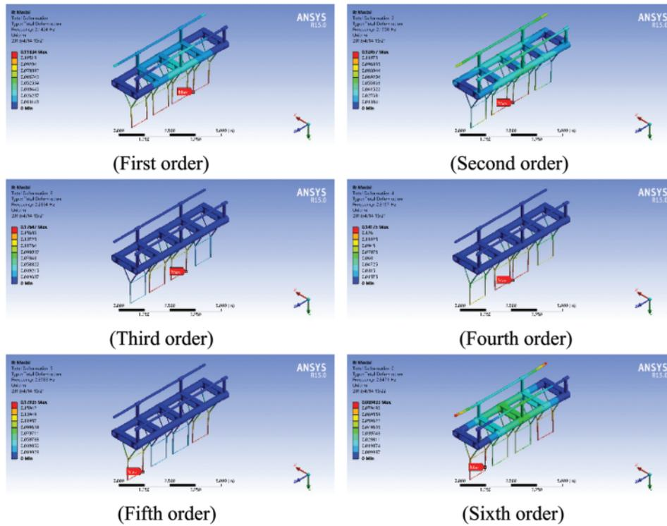
Figure 10: The first six mode shapes of the four units structure
