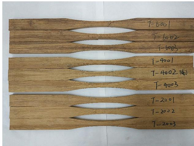
**Figure 7:** Appearance of the bamboo tensile creep specimens
