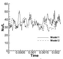
**Figure 8:** Nusselt number Nu/L at  $Ra = 10^8$  using hybrid model 1 (—) and hybrid model 2 (- - - -) using computational mesh 160x80R16
