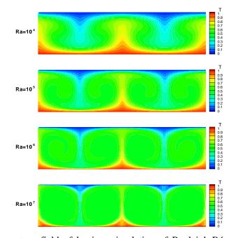
**Figure 2:** Temperature field of laminar simulation of Rayleigh-Bénard Convection on computational mesh  $160 \times 80R16$ . Results are shown from above to below for Rayleigh Numbers  $Ra = 10^4$  (above),  $Ra = 10^5$  (upper middle),  $Ra = 10^6$  (lower middle) and  $Ra = 10^7$  (below).
