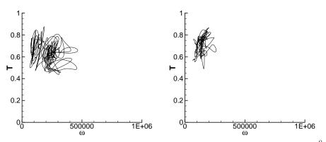
**Figure 4:** Temperature T and vorticity  $\omega$  in point (0.05, 0.04983) at  $Ra = 10^8$  using computational mesh 160x80R16 and hybrid model 1 (figure left) and hybrid model 2 (figure right).
