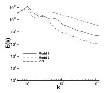
**Figure 10:** One-dimensional longitudinal energy spectrum of turbulence shown for hybrid model 1 (—) and hybrid model 2 (- - - -) using computational mesh 160x80R16 at  $Ra = 10^8$ . Line (- · - · - · -) shows -5/3 slope, which represent inertial subrange of Kolmogorov hypothesis
