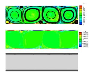
**Figure 6:** Temperature (top), vorticity (middle) and LES/URANS hybrid model area (bottom) field at  $Ra = 10^8$  using hybrid model 1 and computational mesh 160x80R16
