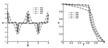
**Figure 3:** Temperature profiles of Rayleigh-Bénard Convection using computational mesh 160x80R16 for the laminar steady-state simulations for Rayleigh numbers from  $Ra = 10^4$  to  $Ra = 10^7$  at height y = H/2 and length x = L/2 respectively.
