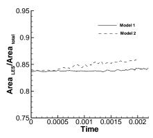
**Figure 9:** The ratio of the area, where SGS model was used in LES/URANS hybrid turbulence model. Hybrid model 1 (—) and hybrid model 2 (- - - -) using computational mesh 160x80R16 at  $Ra = 10^8$
