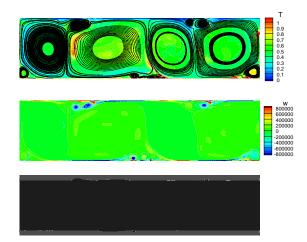
**Figure 7:** Temperature (top), vorticity (middle) and LES/URANS hybrid model area (bottom) field at  $Ra = 10^8$  using hybrid model 2 and computational mesh 160x80R16
