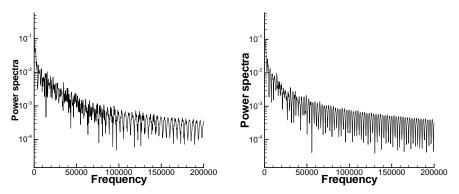
**Figure 5:** Power spectra of temperature time series at point A (0.050, 0.4983) using computational mesh 160x80R16 and hybrid model 1 (figure left) and hybrid model 2 (figure right).
