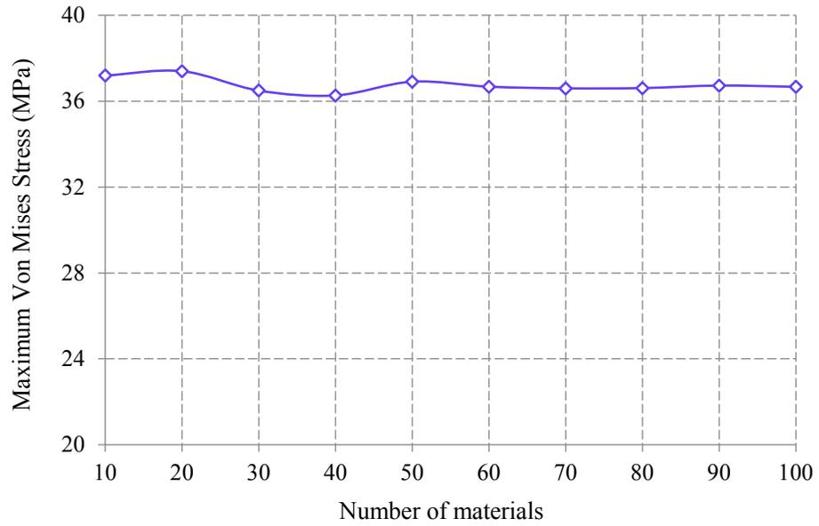
Figure 6: Convergence of the maximum von Mises stress at the femoral neck with the material bins
