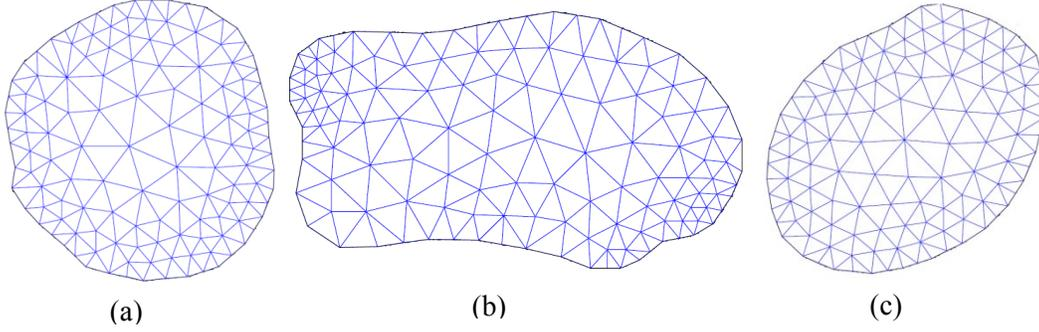
**Figure 4:** Generated triangle elements over (a) the smallest femoral neck cross-section, (b) the intertrochanteric cross-section, and (c) the subtrochanteric cross-section
