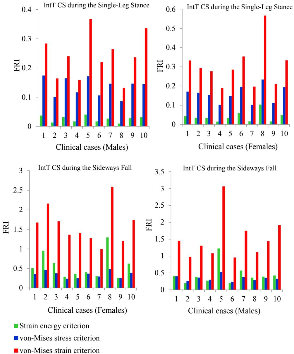
**Figure 11:** Hip fracture risk index (FRI) at the intertrochanteric cross-section of femur (IntT CS) for 10 females and 10 males during the single-leg stance and the sideways fall configurations using the strain energy, von Mises stress, and von Mises strain criteria. (Color should be used for this figure)
