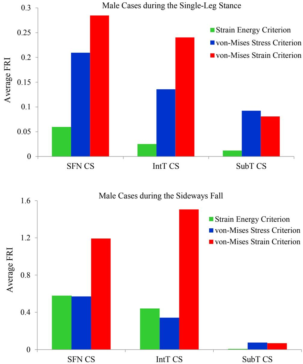
**Figure 14:** Average FRI at the smallest femoral neck cross-section (SFN CS), the intertrochanteric cross-section (IntT CS), and the subtrochanteric cross-section (SubT CS) of femur for 10 males during the single-leg stance and the sideways fall configurations using the strain energy, von-Mises stress, and von-Mises strain criteria. (Color should be used for this figure)
