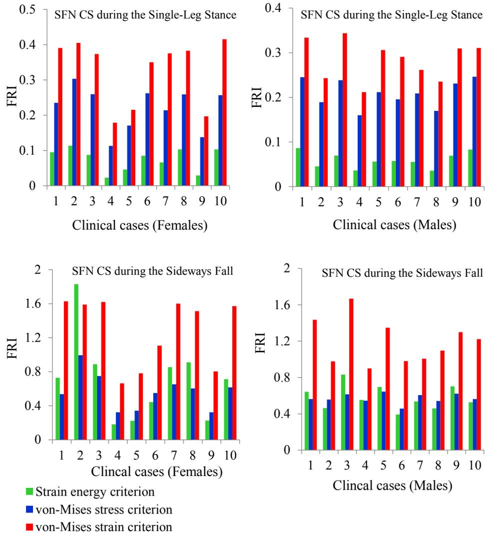
**Figure 10:** Hip fracture risk index (FRI) at the smallest cross-section of the femoral neck (SFN CS) for 10 females and 10 males during the single-leg stance and the sideways fall configurations using the strain energy, von Mises stress, and von Mises strain criteria. (Color should be used for this figure)
