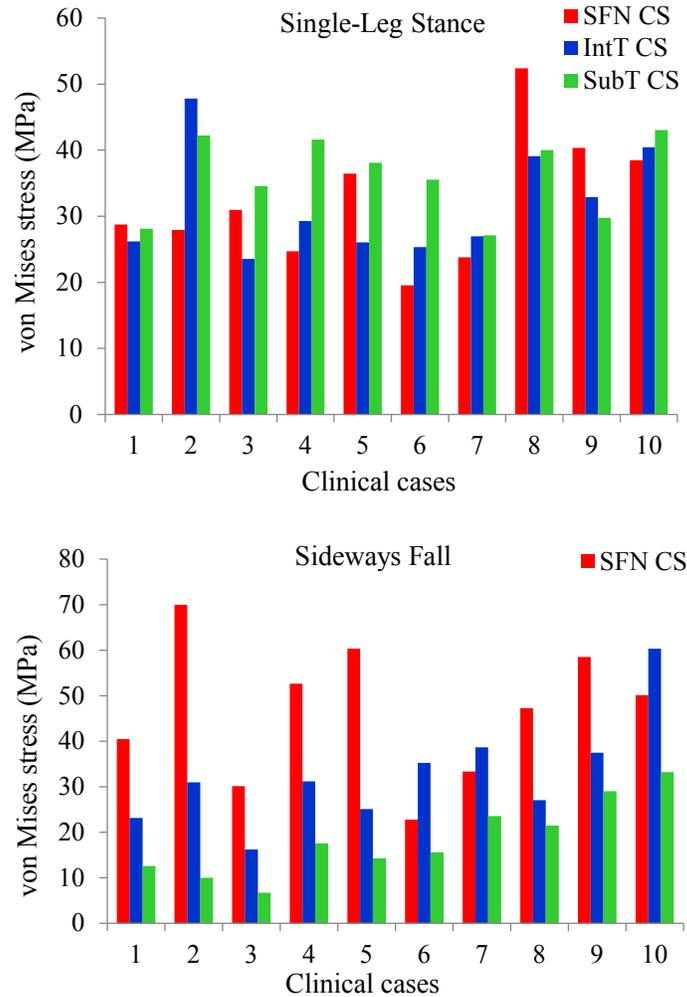
**Figure 8:** Maximum von Mises stress (MPa) at the smallest femoral neck cross-section (SFN CS), the intertrochanteric cross-section (IntT CS), and the sub-trochanteric cross-section (SubT CS) of the femur for 10 clinical cases during the single-leg stance and the sideways fall. (Color should be used for this figure)
