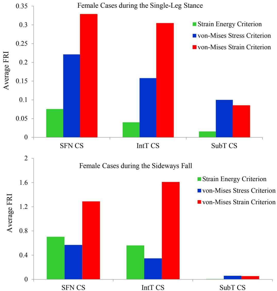
**Figure 13:** Average FRI at the smallest femoral neck cross-section (SFN CS), the intertrochanteric cross-section (IntT CS), and the subtrochanteric cross-section (SubT CS) of femur for 10 females during the single-leg stance and the sideways fall configurations using the strain energy, von-Mises stress, and von-Mises strain criteria. (Color should be used for this figure)
