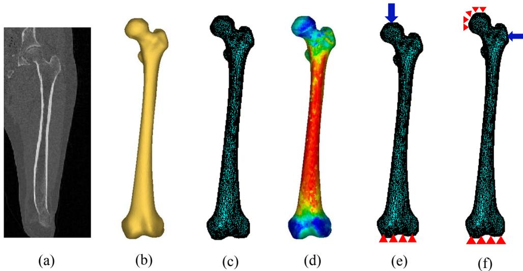
**Figure 2:** QCT-based finite element analysis of the femur: (a) QCT-scan of the femur; (b) 3D model constructed from the QCT image; (c) 3D finite element model; (d) inhomogeneous isotropic material properties assignment; (e) single-leg stance configuration; and (f) sideways fall configuration. (Color should be used for this figure)
