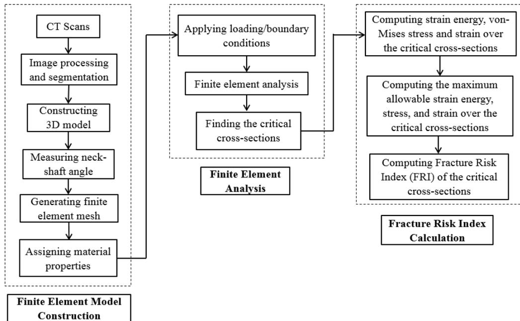
**Figure 1:** The proposed methodology for calculating hip fracture risk index using the strain energy, von Mises stress, and von Mises strain criteria
