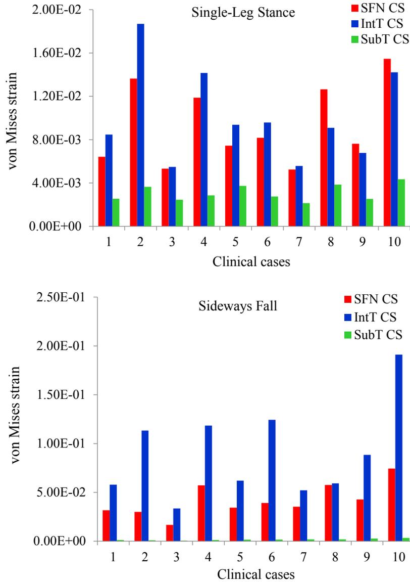
**Figure 9:** Maximum von-Mises strain at the smallest femoral neck cross-section (SFN CS), the intertrochanteric cross-section (IntT CS), and the sub-trochanteric cross-section (SubT CS) of the femur for 10 clinical cases during the single-leg stance and the sideways fall. (Color should be used for this figure)
