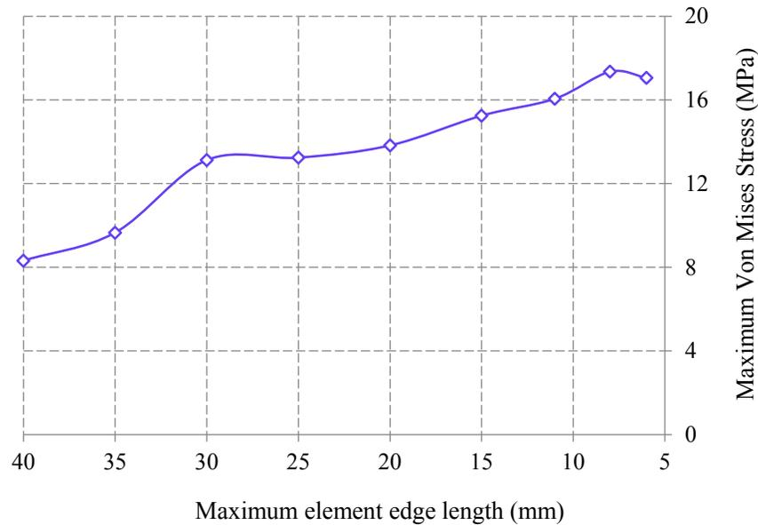
**Figure 5:** Convergence of the maximum von Mises stress at the femoral neck with element size
