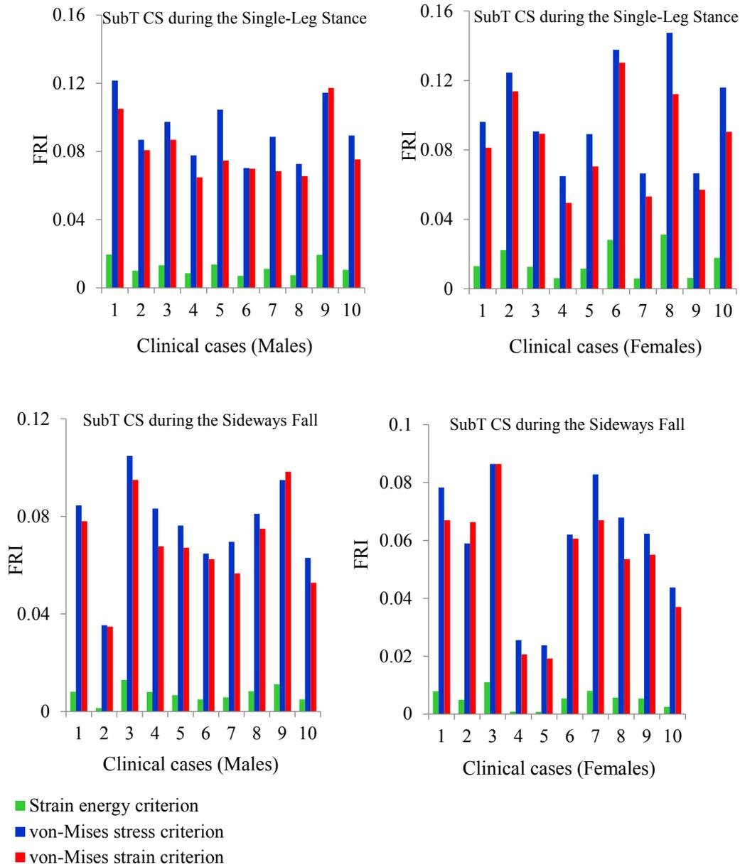
**Figure 12:** Hip fracture risk index (FRI) at the subtrochanteric cross-section of femur (SubT CS) for 10 females and 10 males during the single-leg stance and the sideways fall configurations using the strain energy, von-Mises stress, and von-Mises strain criteria. (Color should be used for this figure)
