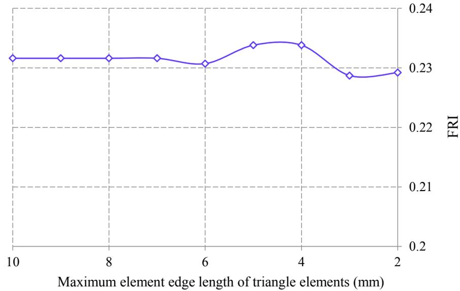
Figure 7: Convergence of the fracture risk index (FRI) with the maximum element edge length of triangle elements generated over the smallest cross-section of femur
