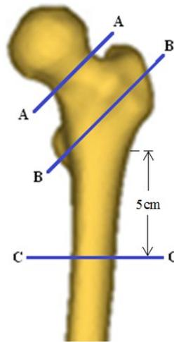
**Figure 3:** Critical femoral cross-sections: the smallest femoral neck cross-section (A-A), the intertrochanteric cross-section (B-B), and the subtrochanteric cross-section (C-C)
